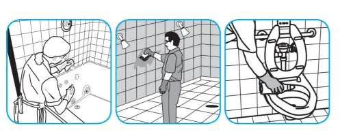
Fill small bottle or bucket or use gun to apply a foam directly onto surfaces. Scrub with a soft brush, pad or cloth. Do not allow foam to dry. Rinse surfaces thoroughly.
