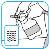
Turn Selector Knob to the high spray position. Spray drain for 2-10 seconds, based on drain size. Allow to stand for up to 30 seconds. Turn Selector Knob to the rinse position. Thoroughly rinse drain.
