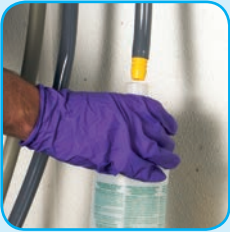
Spray Bottles • Insert spray bottle fill tube into bottle • Push back on yellow activation bar to dispense • Move bottle away from unit to stop dispensing • Use properly labeled bottles
