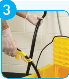
Mop Buckets / Autoscrubbers • Hold long dispensing hose in bucket or clip to side • Pull activation trigger on hose handle to dispense • Lock on with latch for autofill if desired • Release trigger/latch to stop dispensing
