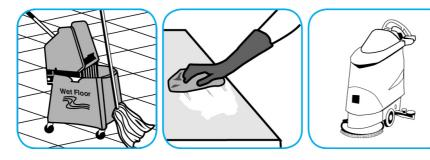
Dilute with cold water. For daily cleaning, use a mop and bucket or fill auto scrubber and use red pads. For Deep Scrubbing, fill auto scrubber and use green or blue pads. Pick-up soil and excess cleaner with a tightly wrung-out cleaning mop.
