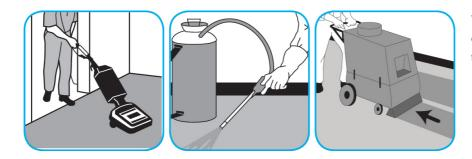
Vacuum carpet first. Fill extractor solution tank with Extraction SC from dispenser. As needed, pre-spot with the appropriate spotter. Extract following equipment maker's operating instructions.
