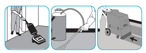
Vacuum carpet first. Fill extractor solution tank with Extraction SC from dispenser. As needed, pre-spot with the appropriate spotter. Extract following equipment maker's operating instructions.
