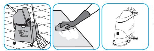
Fill mop bucket, spray bottle or automatic scrubbing machine from dispenser. Apply to surfaces to be cleaned. For auto scrubber use, trail mop behind machine to pick up any excess solution. Allow to dry.
