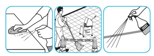
Fill mop bucket, spray bottle or automatic scrubbing machine from dispenser. Apply to surfaces to be cleaned. Allow to dry. For Carpet Spotting: Apply to carpet spot, agitate and rinse with water. For Prespray Cleaning: Apply product to area to be cleaned using a pressurized hand held sprayer. Extract thoroughly with water.
